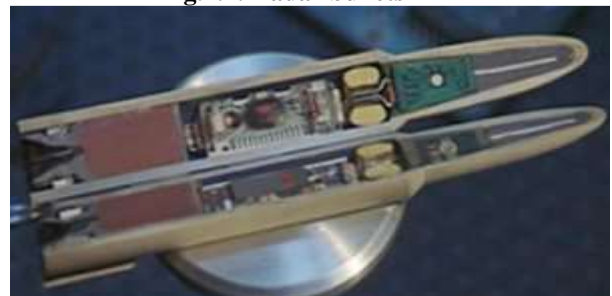
Fig2.3 Internal Structure of Radar bullet
